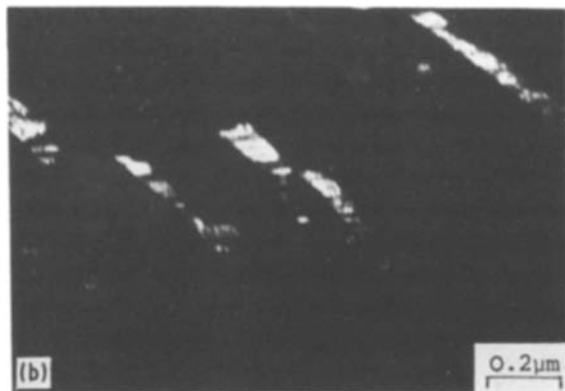
Figure 11 Transmission electron micrographs of \theta' , S' , T_1 precipitates in Al-3Cu-1.5Li-1Mg annealed for 5 h at 250°C; (a) dark-field image of \theta' precipitates with corresponding diffraction pattern showing superimposed [001]_{\alpha} and [001]_{\theta'} zones, (b) dark-field image of S' precipitates with corresponding diffraction pattern showing superimposed [\bar{1}12]_{\alpha} and [101]_{S'} zones.
